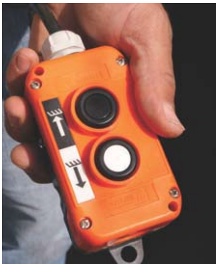
The guys ran an industrial-strength dump-insert control wired to a 16-foot cable into the cab. The cable's long enough for the operator to walk to the end of the vehicle to watch the bed work.
