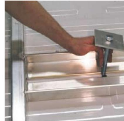
TruckCraft dump inserts use only two 5/8-inch-diameter grade-5 bolts to hold them in place. Both go through major portions of the pickup-truck-bed frame section. While the insert isn't going anywhere, it's easy to remove should the need arise.
