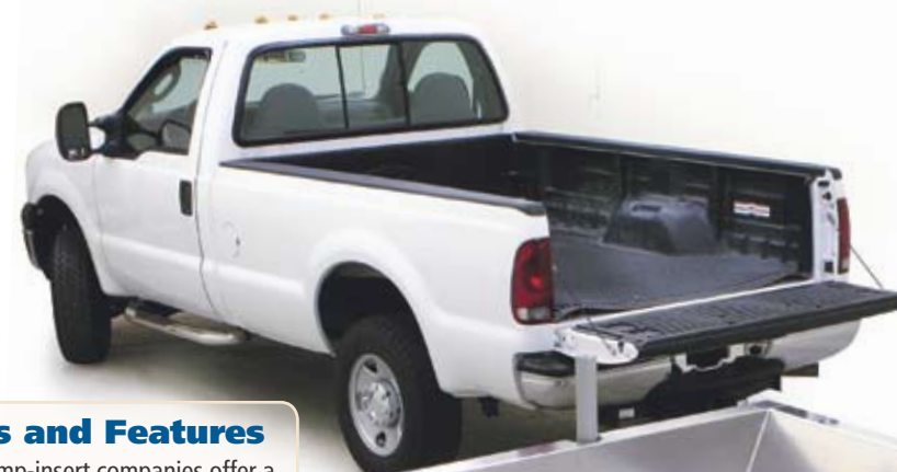
TruckCraft dump inserts use only two 5/8-inch-diameter grade-5 bolts to hold them in place. Both go through major portions of the pickup-truck-bed frame section. While the insert isn't going anywhere, it's easy to remove should the need arise.
