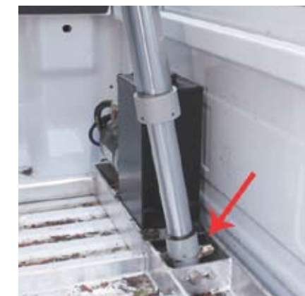
Allowing wood chips, rocks, and other debris to build up is the most common reason for premature hydraulic-ram problems. Keep the area around the ram free of these non-compressible items.
