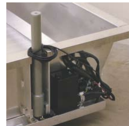
The real magic of these compact workhorses is the small yet powerful hydraulic pump and cylinder systems that lift the dump bed up. The TC-120 Ultra insert can lift 7000 pounds to 47 degrees in 18 seconds.
