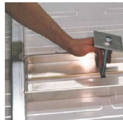
TruckCraft dump inserts use only two 5/8-inch-diameter grade-5 bolts to hold them in place. Both go through major portions of the pickup-truck-bed frame section. While the insert isn't going anywhere, it's easy to remove should the need arise.
